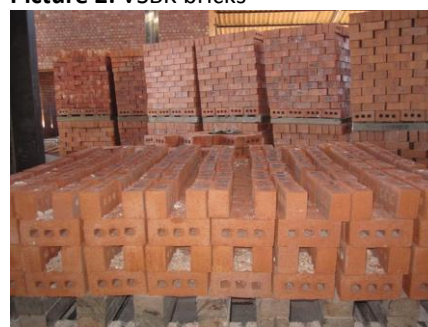
Picture 2: VSBK bricks
