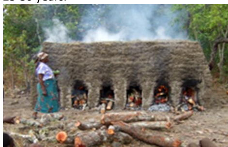
Picture 1: A brick kiln, which is burnt for 24 hours
