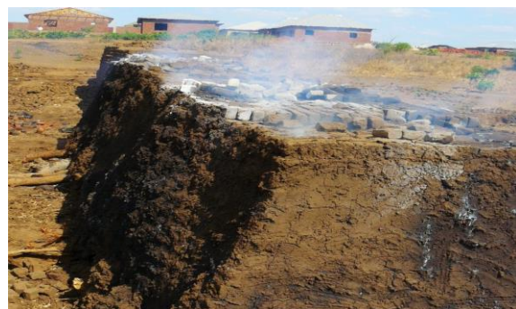
Figure 4: Brick kiln using Wood logs
