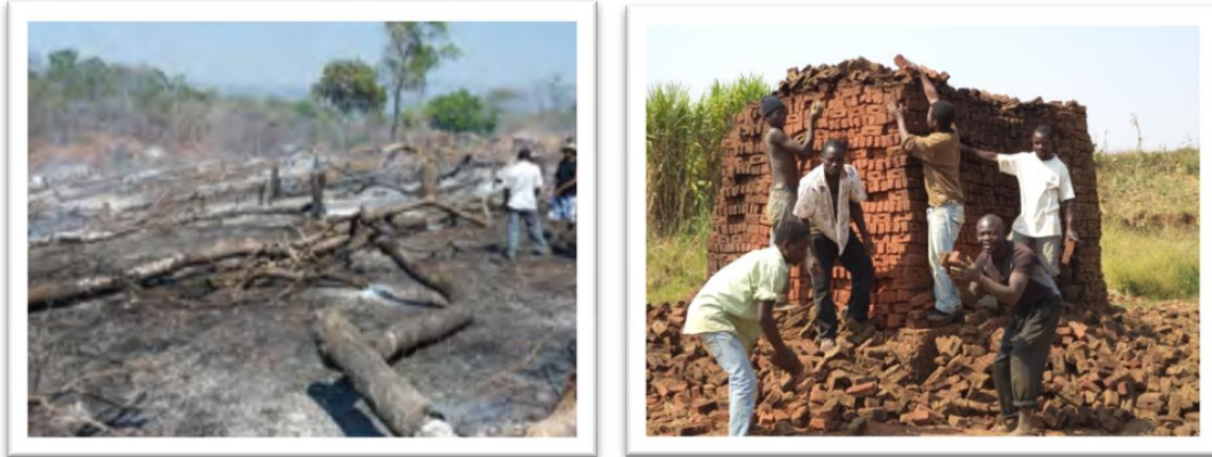
FIGURE 3: LARGE SCALE DEFORESTATION TO FIRE BRICKS (LEFT); WOOD FIRED CLAMP (RIGHT)
