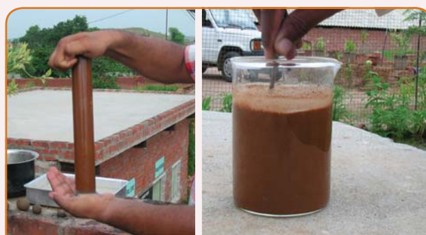
Figure 7: Sedimentation Test for Determining Suitability of Soil for Use in Brick Making
