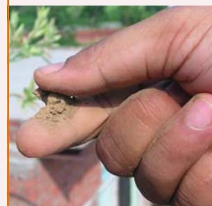
Figure 9: Crumbling Test for Determining Suitability of Soil for Use in Brick Making
