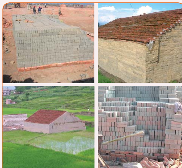
Figure 25: Storage of Green Bricks
