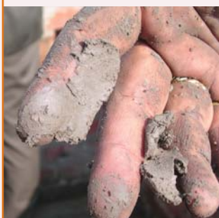
Figure 8: Smearing Test for Determining Suitability of Soil for Use in Brick Making
