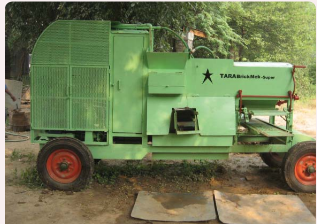
Figure 22: Soft Mud Moulding Machine
