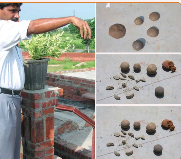
Figure 6: Ball Test for Determining Suitability of Soil for Use in Brick Making
