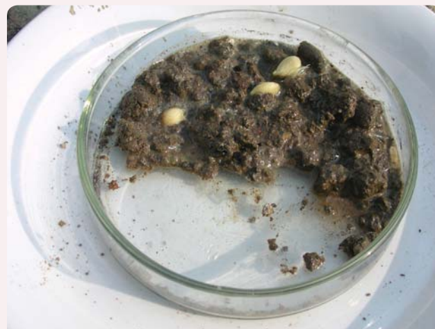
Figure 12: Lemon Test for Determining Suitability of Soil for Use in Brick Making
