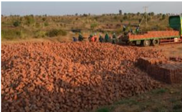
Figure 5: High fired brick breakage due to poor green brick quality
