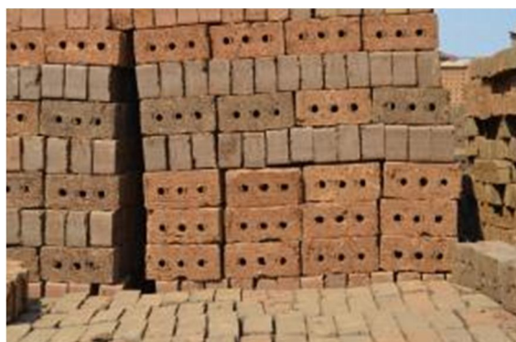
Figure 3: 25mm hollow bricks being produced
