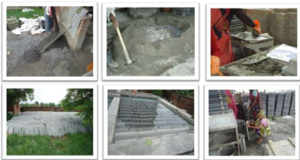
Figure 9: Top Row : Sieving aggregate (left), Mix preparation (centre), Making tiles in moulds (right) ; Bottom Row : Stacking tiles (left), Curing tiles in water tank (centre), Edge cleaning of tiles (right)
